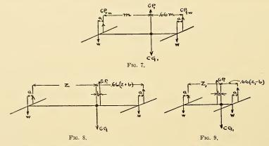
Figs. 7-9. Diagrams illustrating formulæ for moving C. P. without disturbing C. G.
